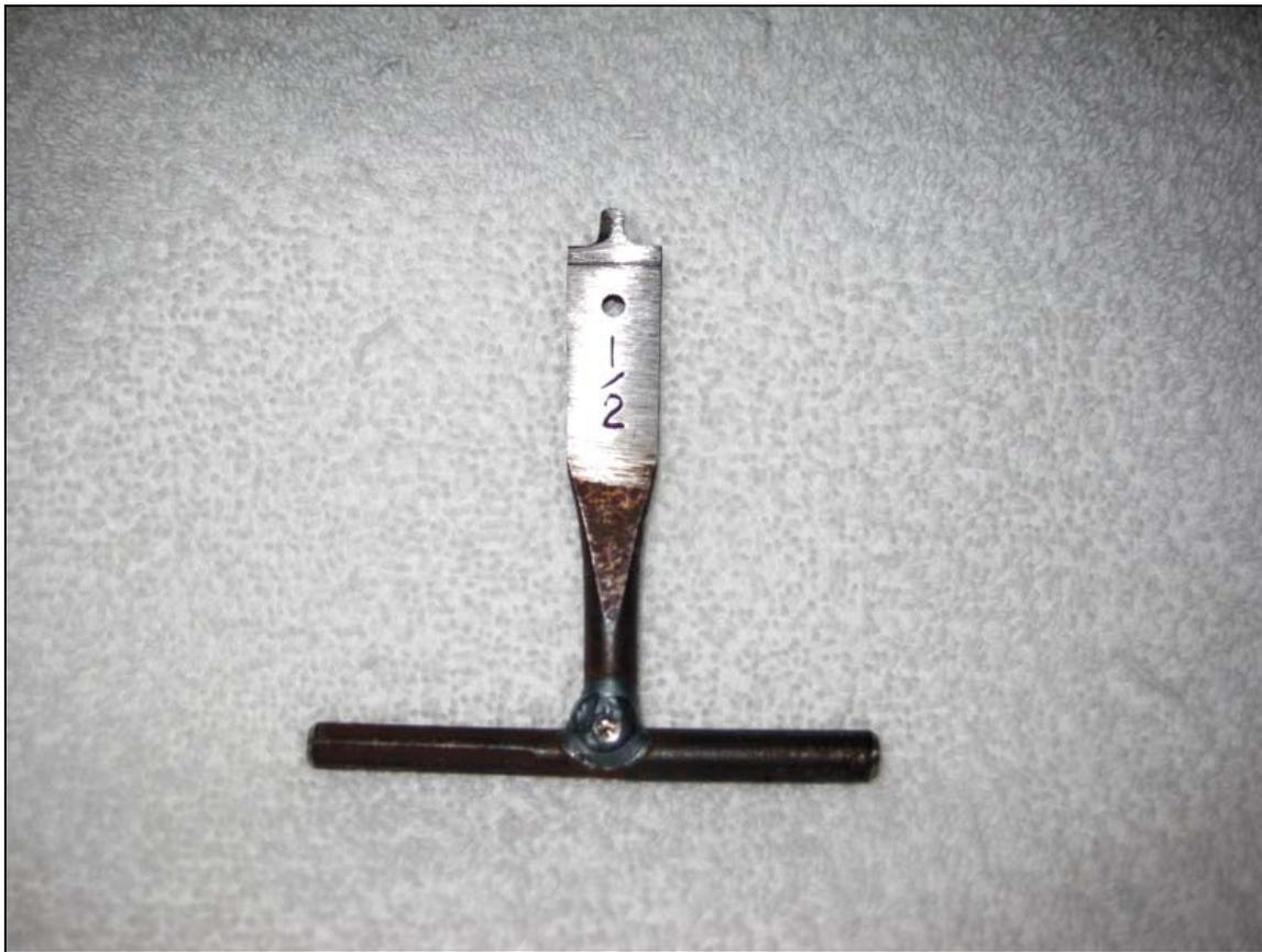
I ground down the cutter point on the spade bit, leaving a stub to center the tool in the needle seat. Then I filed the tip down so that it would have no taper at all, so it is a push fit in the seat slot. Then I cut off the top 3" of the shank and welded it on as a handle. Nothing fancy but it works like a charm.
