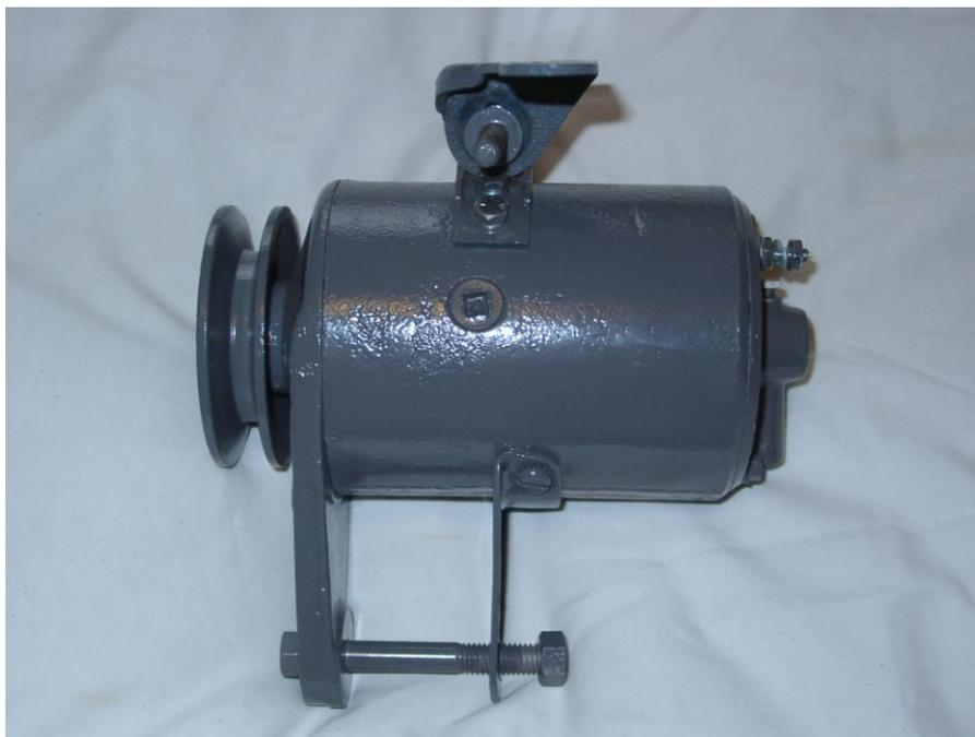
**FIG. 13 –The 2N-10000 Generator & Tensioning Bracket Assembly. Left Side view.**
