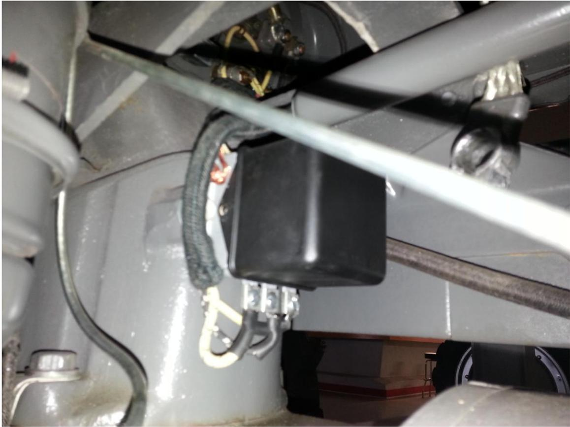
**FIG. 7 –An original 9N-101505 Voltage Regulator mounted correctly. The cast aluminum lower steering box provided two bosses drilled and tapped 5/16-18 NC for hex bolts to secure the unit. Note the downward pointing position of connection tabs. The copper-braided ground strap is secured with the hex bolt on the top left.**
