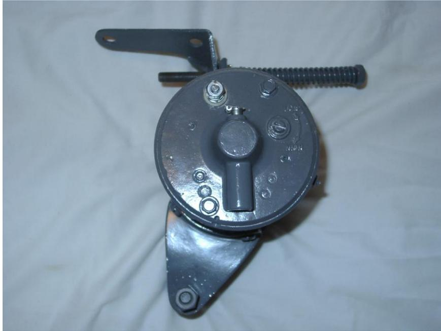
**FIG. 14 –The 2N-10000 Generator & Tensioning Bracket Assembly. Back view.**
