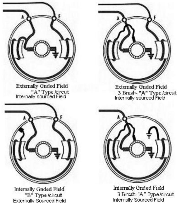
**FIG. 2 –Generator 'A' and 'B' electrical circuits defined.**
