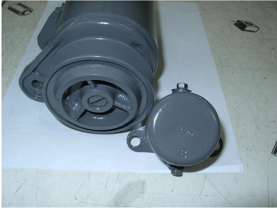
**FIG. 9-A –The original 9N-10000-B Generator with the smaller 9N-10130-D Pulley and an original 9N-10505-B Cutout.**
