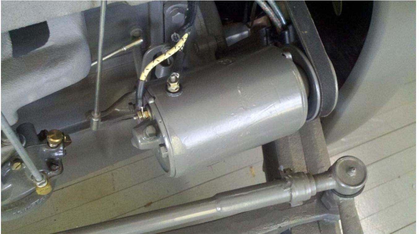
**FIG. 3 –Early 9N-10000 Generator -a 2-wire/2-brush, B-Circuit design. Output rated at 7 amps maximum at 7.5 volts constant. After the 9N-10000-B generator was released, the original was designated with the 'A' suffix.**
