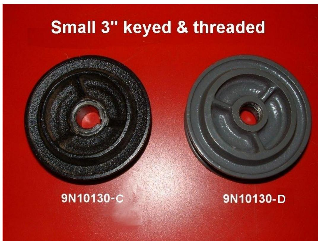
**FIG. 10 –The smaller 9N-10130-C and 9N-10130-D Pulleys. Designed with a smaller Major OD at 3-3/16" and therefore a smaller Over-The Roll\* dimension. Note the 'C' is keyed and replaced the 'A' pulley and the 'D' is threaded which replaced the 'B' pulley.**
