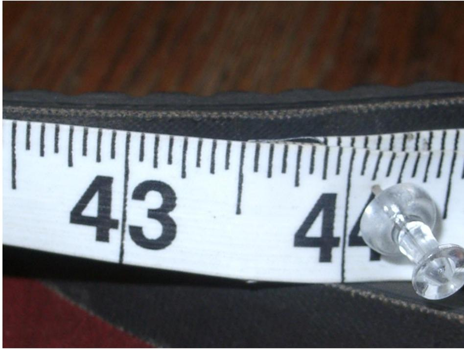
**FIG. 17 –The length of a new 9N-8620-A fan belt is measured at 43-1/2 inches around the outside. Width of belt is 11/16" measured at the outside. Bear in mind a new belt will have stretched so this is not the best method to determine belt length.**
