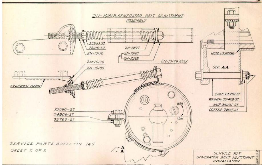
**FIG. 12 –Original drawing for the belt tensioning kit. This was a Service Item sold by dealers and fit the 9N-10000-C Generator.**
