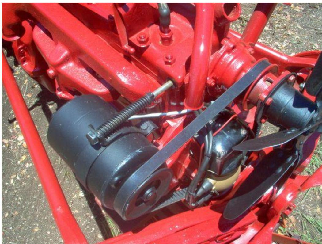
**FIG. 11 -9N-10000-C Generator with the 9N-10130-B, threaded pulley. 1- wire, 3-brush style, rated output at 11.5 amperes. Shown with tensioning bracket kit assembly.**
