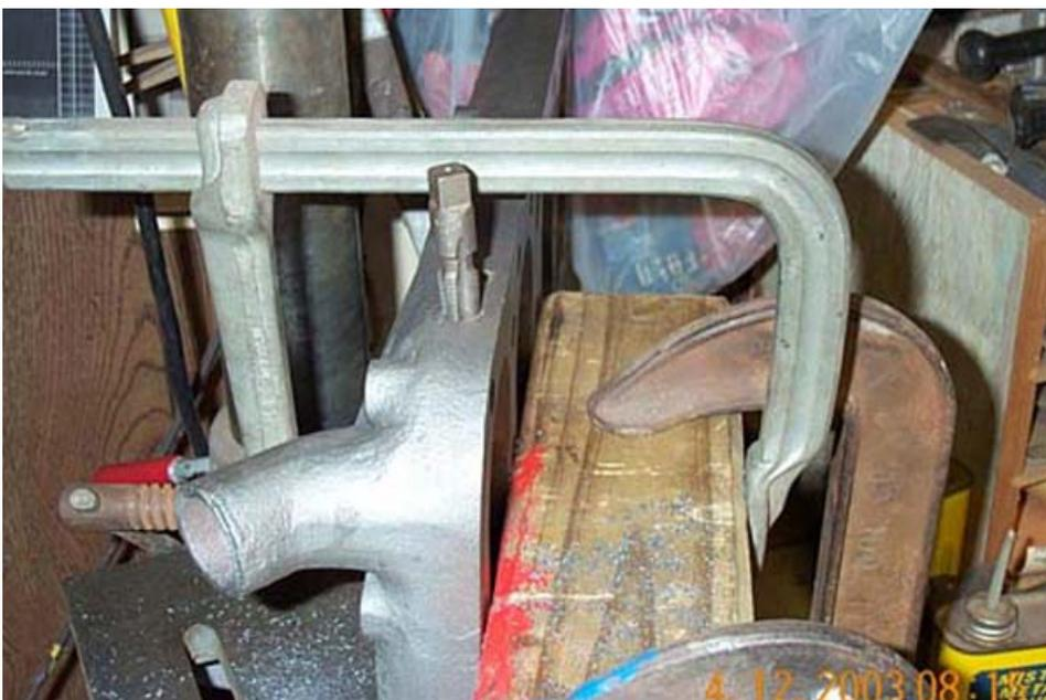
This is the end result. The sensor fits good. The head material is 3/16" to 1/4-inch thick in this spot. The head is set loose on the block. I turned the engine over and watched for any movement of the head, all is well with that, also.
