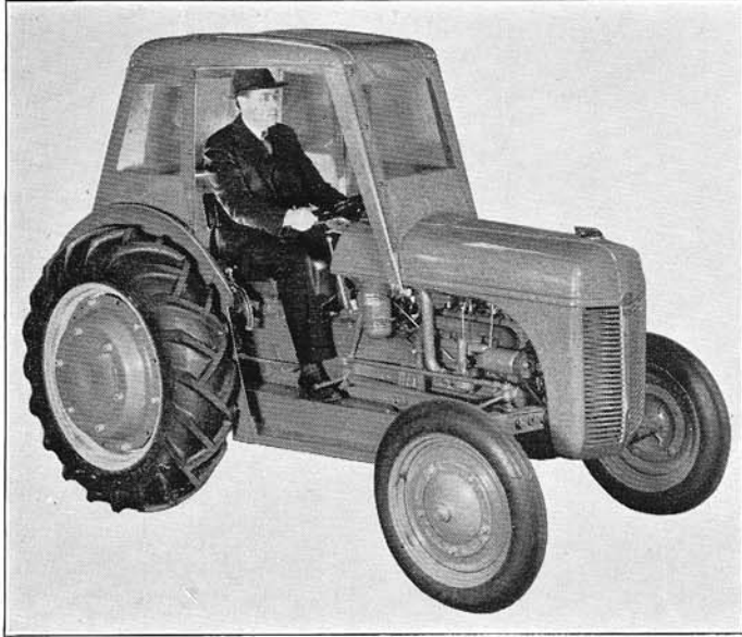
Cab with Door Curtain Removed
