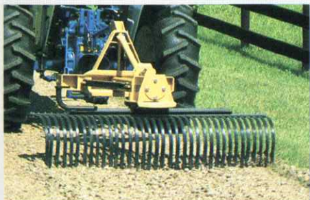
Series 762A landscape rake is available in 72 and 96-inch widths. Seven angle settings right and left, are standard. Flip-down grader blades and single or dual gauge wheels are optional.
