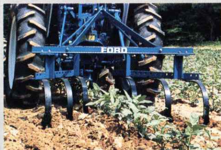
Series 400A cultivator cultivates one row and provides 22½ inches of crop clearance. This mounted cultivator includes six spring shanks with 2-inch reversible shovels.
