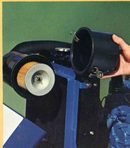
All 1000 Series tractors are equipped with easy-to-service dry air filters.
