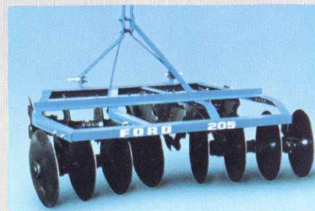
Series 205 economy disc harrow is offered only with 16-inch notched blades front, and plain blades rear. It comes in 53, 67 and 82-inch widths, with 12, 16, and 20 blades, respectively. Scrapers are optional.
