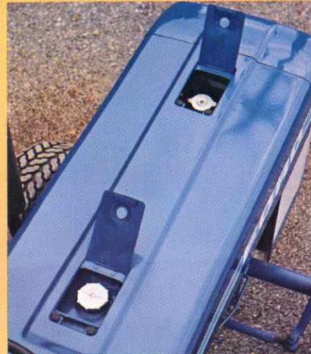
Access doors on most models allow fuel and water to be added without raising the hood.
