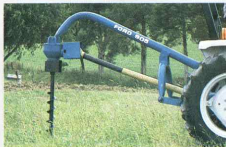
Series 905 posthole digger is rear-mounted, PTO driven, auger-type digger capable of digging holes from four inches to 12 inches in diameter, and up to 42 inches deep.
