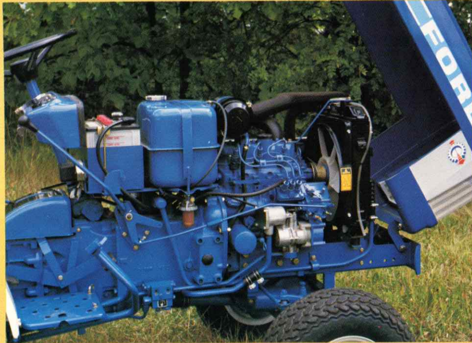
The hood tilts forward for simple servicing of engine, air cleaner and battery.
