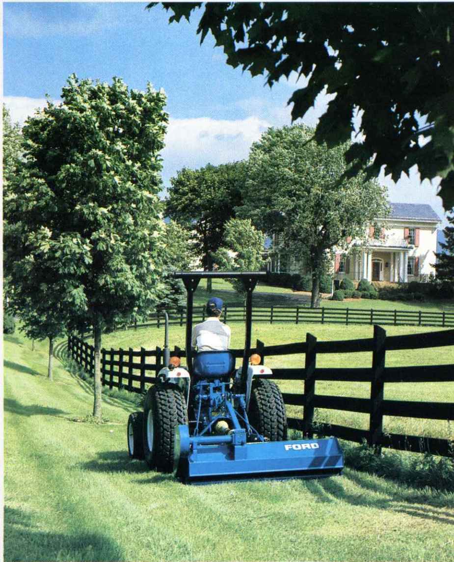
951 Special rotary cutters are available for 1000 Series tractors in 48, 60 and 72-inch widths. Straight bar or Stump Jumper blade carrier. Laminated tire and chain guards are optional.
