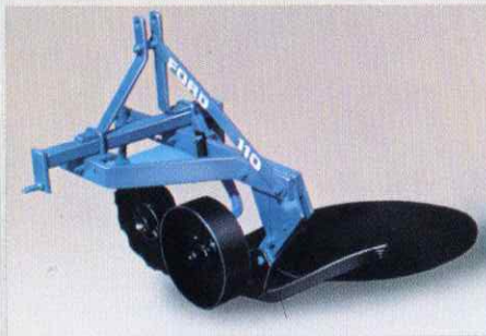
Series 110 economy plows come with one or two bottoms in 12, 14, or 16-inch widths. They have shear bolt beams, landside, 15½-inch coulter, and a gauge wheel.
