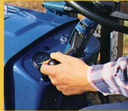
Location of the SMS shift lever frees operator's right hand for steering and hydraulic control.
