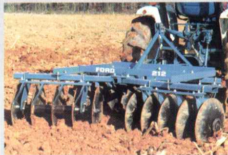
Series 212 mounted disc harrow is available in 65, 78 and 91-inch widths. Gang angles adjust from 5 to 20 degrees. 18-inch blades are notched in front, plain in rear. 7¼-inch blade spacing.
