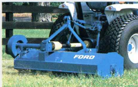
Series 917L flail mowers are light-duty mowers that give a finished cut. Mower blades rotate vertically, cutting is parallel to the ground. Available in 50 and 60-inch cutting widths. Gauge rollers protect the ground.
