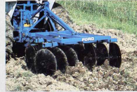
Series 200A economy disc harrow has 16-inch blades with 8-inch spacing. Front blades are notched. Three-point hitch mounted. Available in 52 and 67-inch widths.
