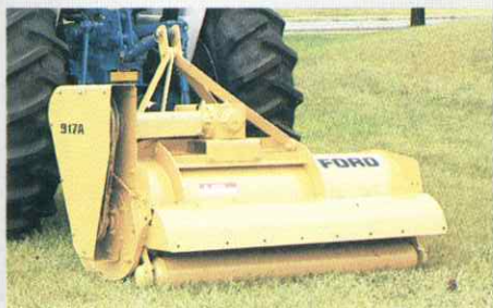
Series 917A flail mower comes in 48, 62 and 74-inch widths. Mower blades rotate vertically with cutting action parallel to the ground. This reduces likelihood of objects being thrown.
