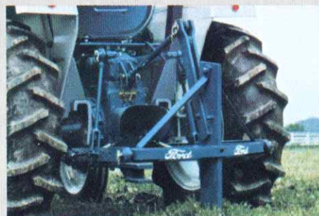
Series 107 subsoiler breaks hardpan to improve water absorption, subsurface drainage, root growth. A ¾ x 18-inch shank and reversible chisel point are standard.
